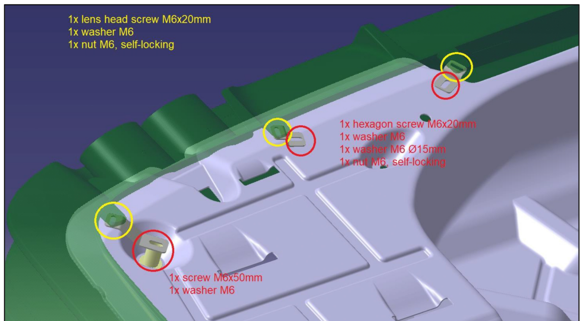
Fig 9: Assignment of fixing materials (left-hand side of vehicle)
