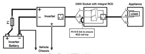
Fig3 - Example RCD installation
