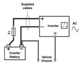
Fig1 - Example single battery system
